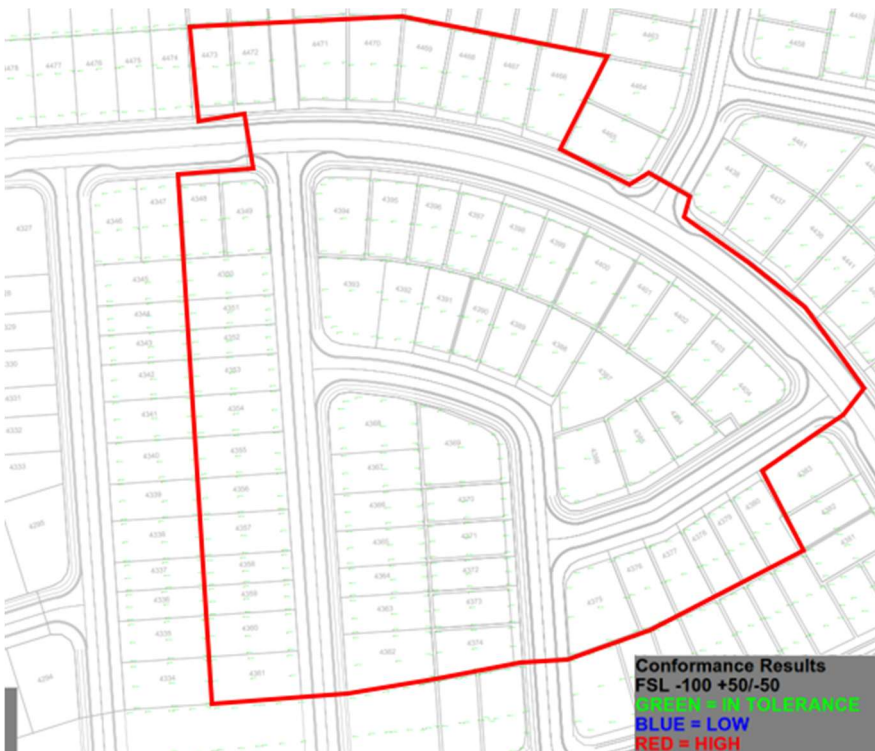
Figure 4: Actual Constructed Area of Fill (100mm BFsL) – Shadforth Survey Plans
