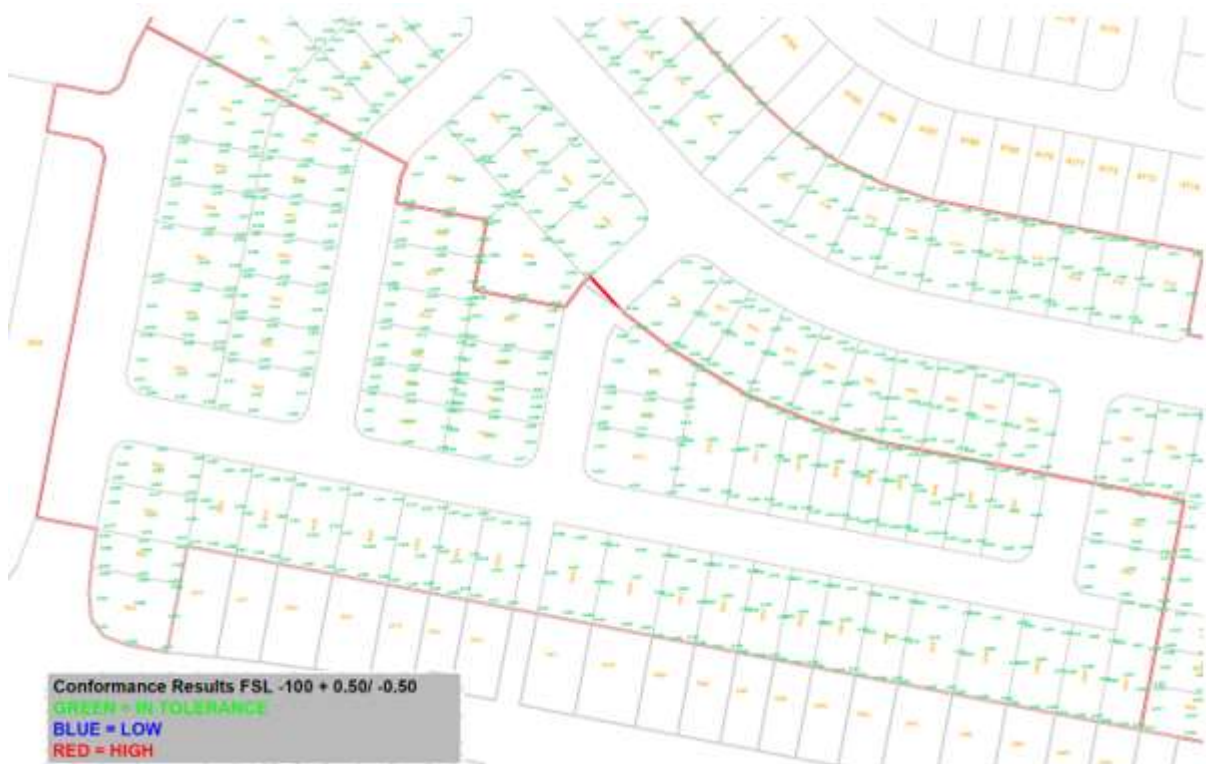
Figure 3: Actual Constructed Area of Fill (100mm BFSL) – Shadforth Survey Plans
