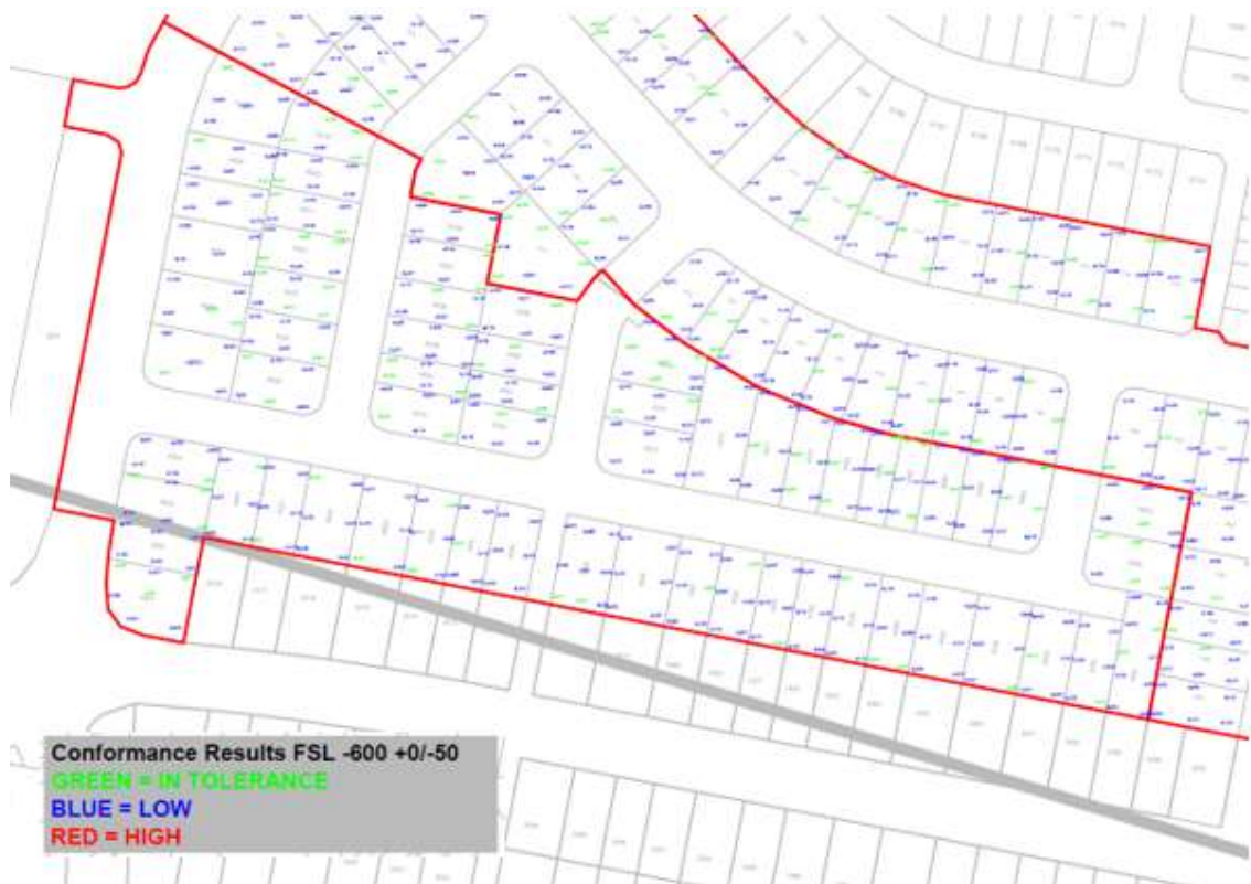
Figure 2: Actual Constructed Area of Fill (600mm BFSL) – Shadforth Survey Plans
