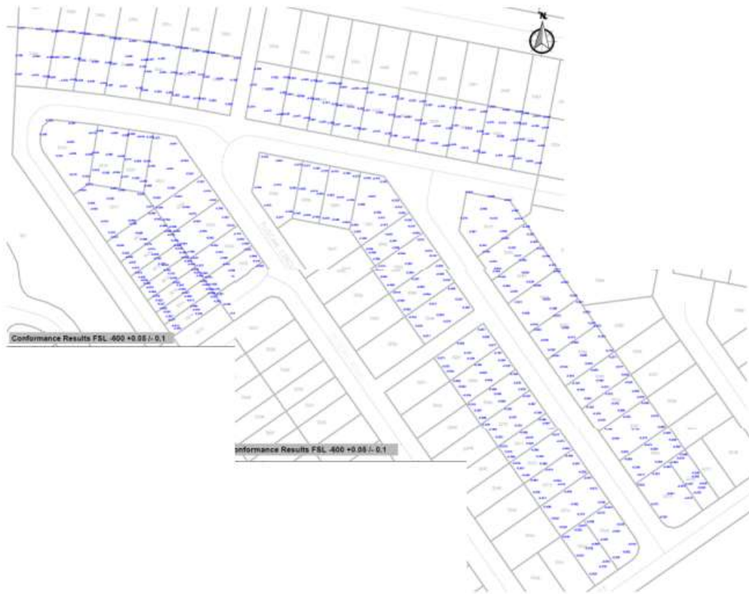
Figure 3A: Actual Constructed Area of Fill (600mm BFSL) – Shadforth Survey Plans
