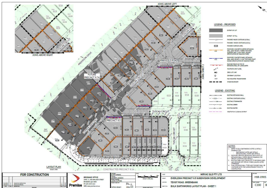
Figure 2: Extent of Fill (Precinct 9.5) - Premise Earthwork Drawing MIR-0905-C201-B
