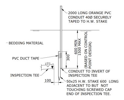
Due to this, when excavated and exposed for connection, this fitting is often displaced. This fitting must be checked and readjusted to ensure fall has been maintained prior to connection. If there is concern backfall might existing in the pipework past the inspection tee, please contact the developer immediately, prior to connection or backfilling so it can be checked and rectified if required.
