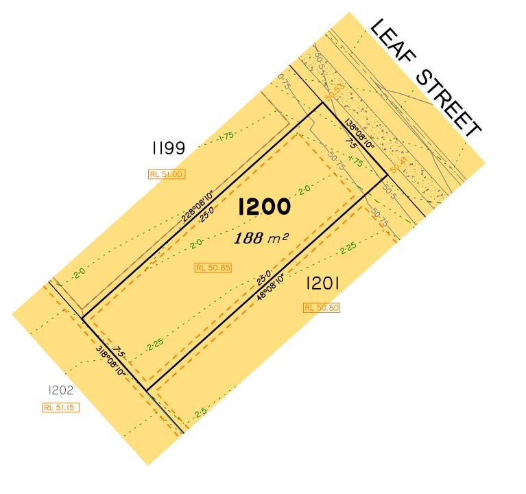
**LEGEND** Area of Fill Area of Cut **Design Contours**  Depth of Fill Contours Retaining Wall Tiered Retaining Wall Proposed Earthworks Pad RL XX.XX Finished Pad Design Level
