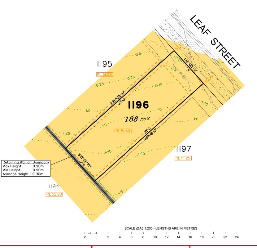
**LEGEND** Area of Fill Area of Cut **Design Contours** - Depth of Fill Contours Retaining Wall Tiered Retaining Wall Proposed Earthworks Pad RL XX.XX Finished Pad Design Level XX.XX Finished Surface Design Level
