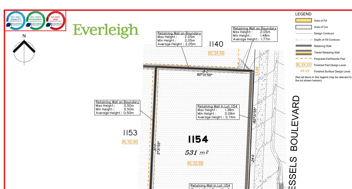
Retaining Wall on Boundary (Front of Lot Transition) Max Height: 0.5m 0.00m Min Height : Average Height: 0.25m
