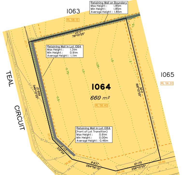
**LEGEND** Area of Fill Area of Cut **Design Contours** - Depth of Fill Contours Proposed Retaining Wall Proposed Tiered Retaining Wall Proposed Earthworks Pad RL XX.XX Finished Pad Design Level XX.XX Finished Surface Design Level (Not all items in this legend may be relevant to
