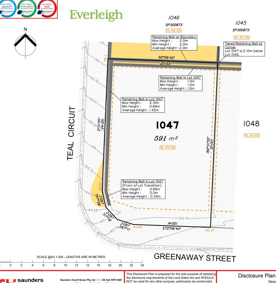
**LEGEND** Area of Fill Area of Cut **Design Contours** - Depth of Fill Contours Proposed Retaining Wall Proposed Tiered Retaining Wall Proposed Earthworks Pad RL XX.XX Finished Pad Design Level XX.XX Finished Surface Design Level (Not all items in this legend may be relevant to
